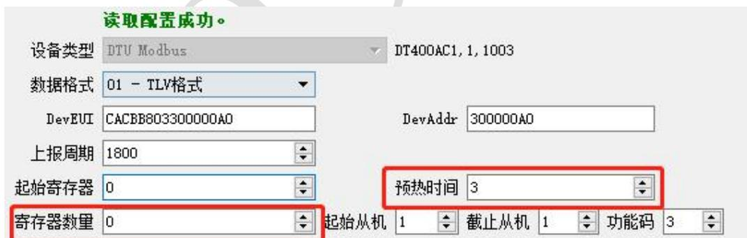
The screenshot shows the SensorTool configuration window with non-Modbus settings. The '通用' section contains the following fields: '设备类型' (DTU Modbus), '数据格式' (01 - TLV格式), 'DevEUI' (CACBB803300000A0), 'DevAddr' (300000A0), '上报周期' (1800), '起始寄存器' (0), '寄存器数量' (0), '预热时间' (3), '起始从机' (1), '截止从机' (1), and '功能码' (3). The '起始寄存器' and '寄存器数量' fields are highlighted with a red box. At the bottom, there are buttons for '读配置', '更新配置', and '重启设备'.
